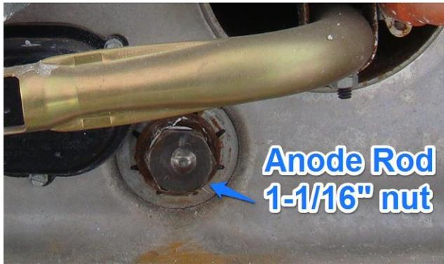
The water in the tank creates a chemical reaction that can attack and destroy the lining of the water heater. In order to protect the lining, a sacrificial anode rod is used. As the rod is worn away, it will eventually need to be replaced. A new anode rod costs about \$15, is available at most RV dealers, and from numerous online sellers, and can be installed without any special training. You will need a 1-1/16" socket to remove the old rod.
