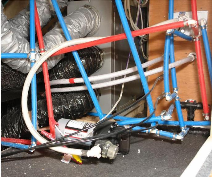
The water pump is located on the floor behind the UDC. When winterizing, the pump will suck antifreeze in and pump it through the water system (but not into the fresh tank or through the black tank flush systems). However, if using compressed air to winterize, you must take additional steps to protect the water pump and its filter assembly. Consult our [Winterization Guide](#) for details.
