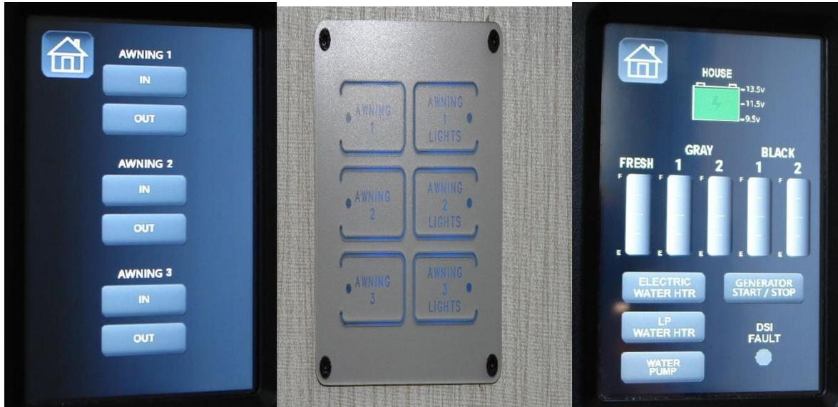
KIB Awning Control Screen, Awning Local Switches, Tank and Batter Levels, Water Heater and Pump Controls
