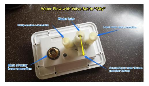
If you disconnect the Fresh water tank connection fitting on the right, along with the Pump suction connection on the left, with city water is turned ON, and the Anderson Valve set to CITY, check for water coming out of the open left and right valve fittings. That would indicate a leaking O-ring or valve seat inside the valve assembly.
