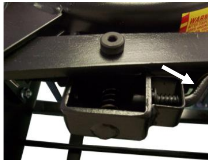
Figure 5.6 Retainer Pin view at Eight o'clock
