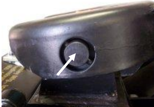
Figure 7.1 Lubricate fore and aft pivot pins
