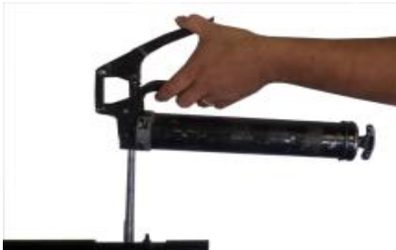
Figure 6.1 Grease every 4,000 miles
