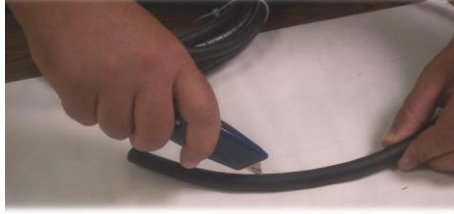
Figure 4.15 Strip the outer jacket
