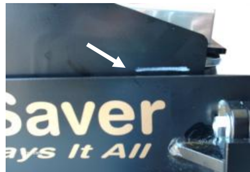
Figure 4.6 Inflating to the white mark
