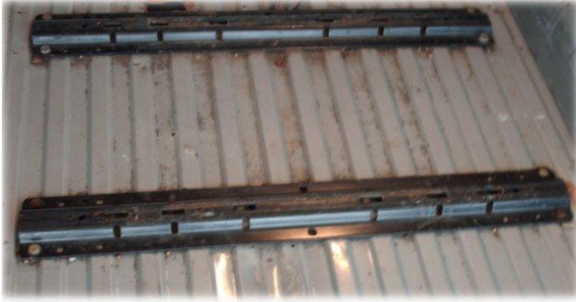
Figure 3.1 Standard top mounted slotted rail
