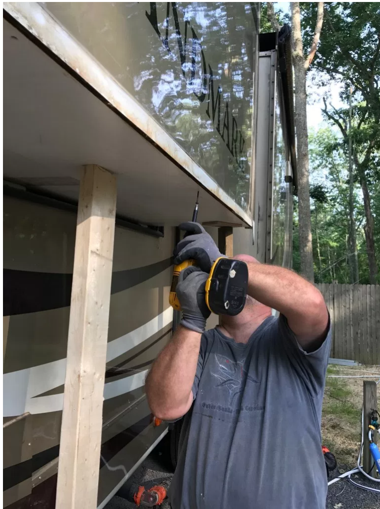
Installing outside perimeter screws while supporting the lap joint with 2 x 4s
