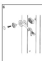
Step 6A). Travel Latch Assembly is factory installed onto left side Wall Jamb. Latch Assembly is factory adjusted to a postion that should hold the Glass Panels tightly. B). Gather Glass Panels to left wall jamb and Latch the Hook onto the Catch. If Glass Panels are not held tightly, Loosen/ Adjust/ Tighten the Travel Latch Assembly as required.
