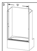
Step 3A). Measure the Finished Opening Width 'B' at the Top of the Enclosure (the installation location). B). If needed, Cut the Header 1/8 inch shorter than measured length.
