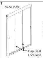
**Step 7.** Install Gap Seals onto the inside edges of Glass Panels, with the soft finger seal reaching toward the outside of the unit.
