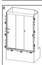
**Step 8.** Apply Clear Silicone on the Outside of the enclosure wherever aluminum meets Pan / Surround. Also, apply Silicone on the Outside at the Connection of the Sill and both Jambs.
