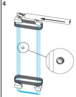
Step 4. Insert Glass Panel Assembly with surrounding packaging material into the Header as shown. (Note: The Travel Latch Catch is on the outside of the Unit.)
