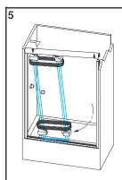
Step 5A). Angle left side of Header onto left Wall Jamb. Slide Panels to the left and lower into Sill channels. Lower right side of Header onto right Wall Jamb.
