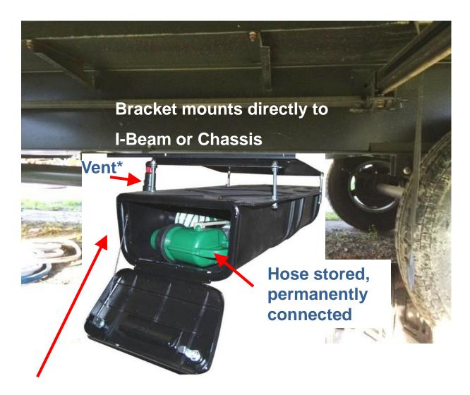
Exit plumbing modified and aligned to enclosure side entry hole. Note the drop height adjustment the bracket kit offers
