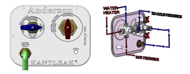
TO FILL STORAGE TANK FROM PRESSURIZED CITY WATER
