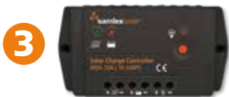
MSK-10A Built-in Charge Controller
