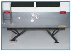
Jacks expand and automatically adjust to the terrain.
