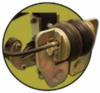
Center Point's simple design cushions the RV against road shock by adding an air bag at the equalizer position between the leaf springs providing smooth, stable towing.
