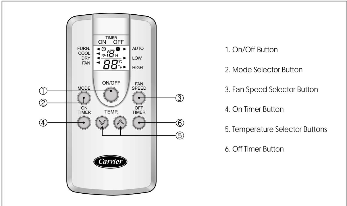
**1 ON/OFF BUTTON** - If you press this button, the unit will begin operation. (You can hear receiving beeps twice.) Press the button again, and operation stops. (You can hear a receiving beep.) If you press this button immediately after turning off the unit, the compressor will not operate for 3 minutes to prevent overloading.
