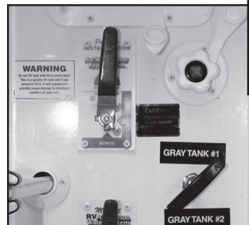
Water Heater Bypass (One Valve System)
