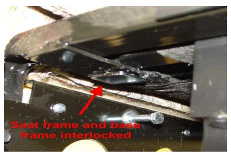
Then reinstall the self-tapping bolts into the seat frame, where you took them out. Roll the air bladder back over the seat cushion. Drape the air bladder motor below the seat cushion and plug the air bladder back in. Make sure there are no objects behind the sofa that could damage the air bladder. Fold the backrest; back up as if are making the bed back into a sofa.
