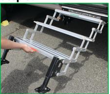
Once **handle** is down, pull from bottom step and extend step to the ground.
