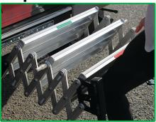
Completely **collapse\* steps** by picking up bottom step and walking in toward the RV.
