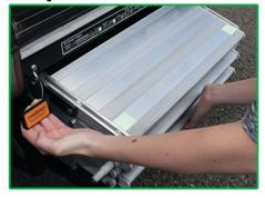
With the steps fully collapsed, lift handle and **rotate steps** up and inward while guiding the guide pins into the guide slots located on both sides of the mounting cage until step stores into place in the stored position.
