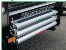
As steps roll in, release the handle. When the handle drops into place, reattach **safety pin** to secure steps.
