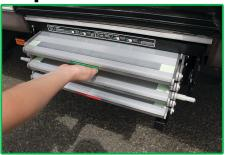
With handle lifted, pull from top step, as step rolls out, release lever to allow lever to automatically drop into the no. 1 (highest) step position.
