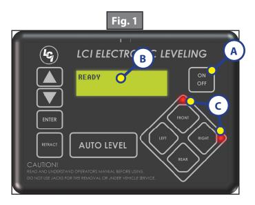
**3.** Push the DOWN ARROW to scroll to "DROP FRONT JACKS" option on LCD screen.
