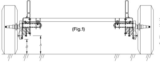
Step 1: Dim. A – Dim. B = C Step 2: Deflection = 5-C
