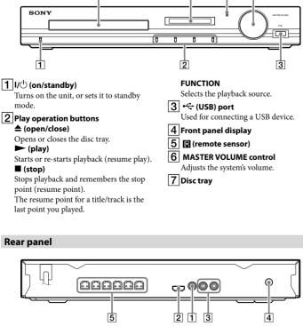
**1** VIDEO OUT jack 4 ANTENNA (FM COAXIAL 75Ω) jack 2 HDMI OUT jack 5 SPEAKERS jacks **3** TV/CABLE (AUDIO IN L/R) jacks
