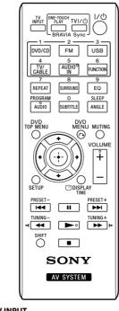
TV INPUT Switches the TV's input source between the TV signal and other input sources. BRAVIA Sync ONE-TOUCH PLAY Activates One-Touch Play TV I/🖰 (on/standby) Turns on the TV or sets it to standby mode.
