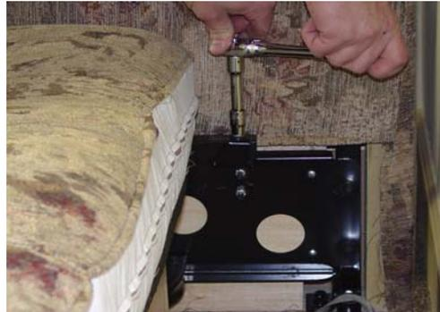
When the bolts are removed, put the backrest in sofa position. Then slide the seat cushion back then lift seat cushion frame up and pull towards the front and out of the sofa.
