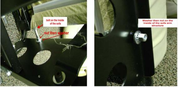
Make sure that the bolt is tighten firmly and is straight.
