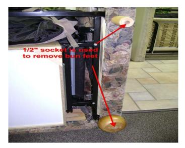
Then, <u>for all sofas</u>, remove the 10 silver Phillips screws, and the arm should slide outward and off the metal structure.
