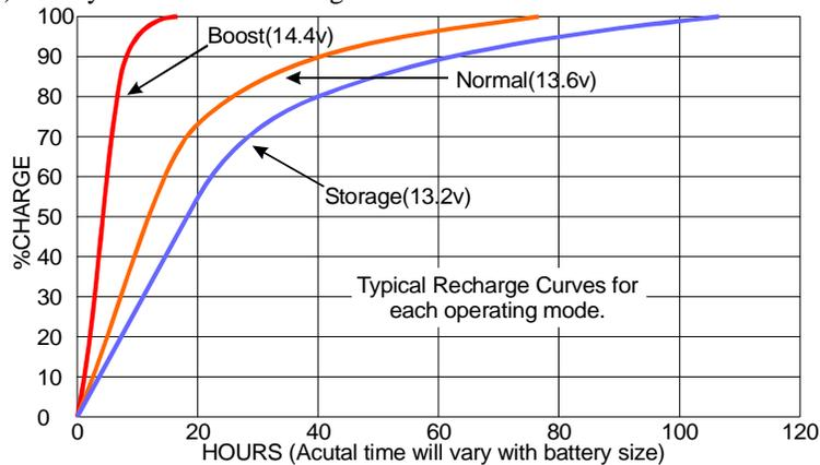
**14.4 Volts (Boost Mode)** – Returned the battery to 90% of full charge in approximately 8 hours. The battery reached full charge in approximately 11 hours.
