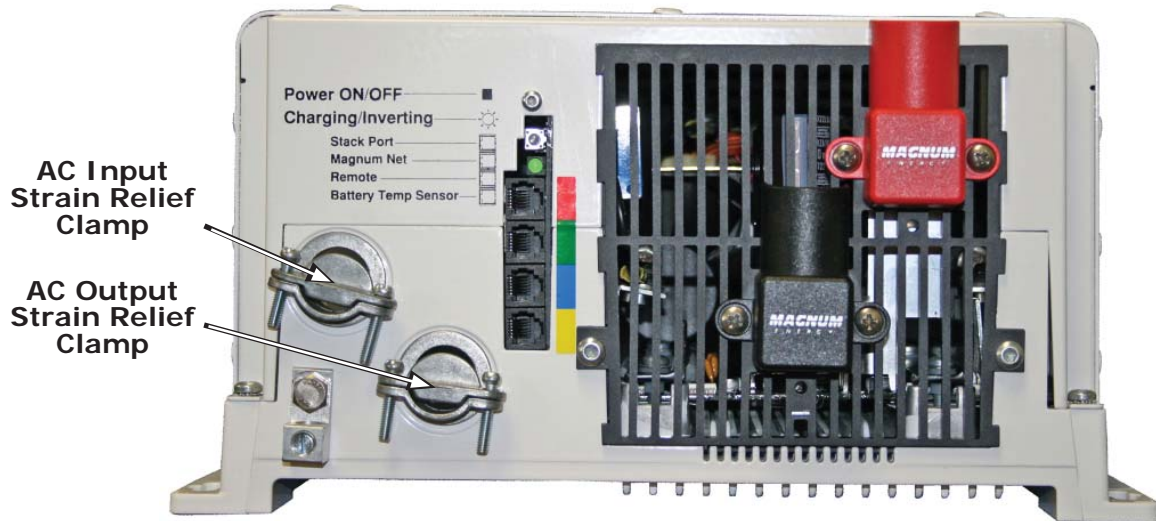
Figure 2-8, MS Series Inverter/Charger - AC Wiring
