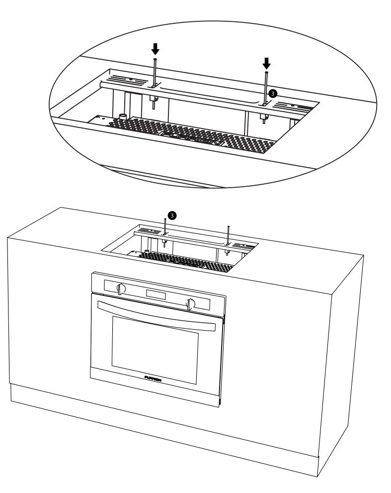
STEP 6 - Mount the vent cover over the vent
