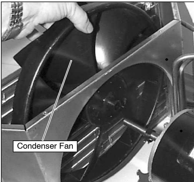
Figure 3-23 Condenser Fan Removal
