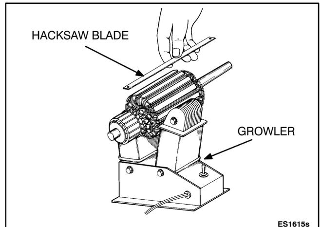
FIGURE 8-20. TESTING ARMATURE FOR SHORTS
