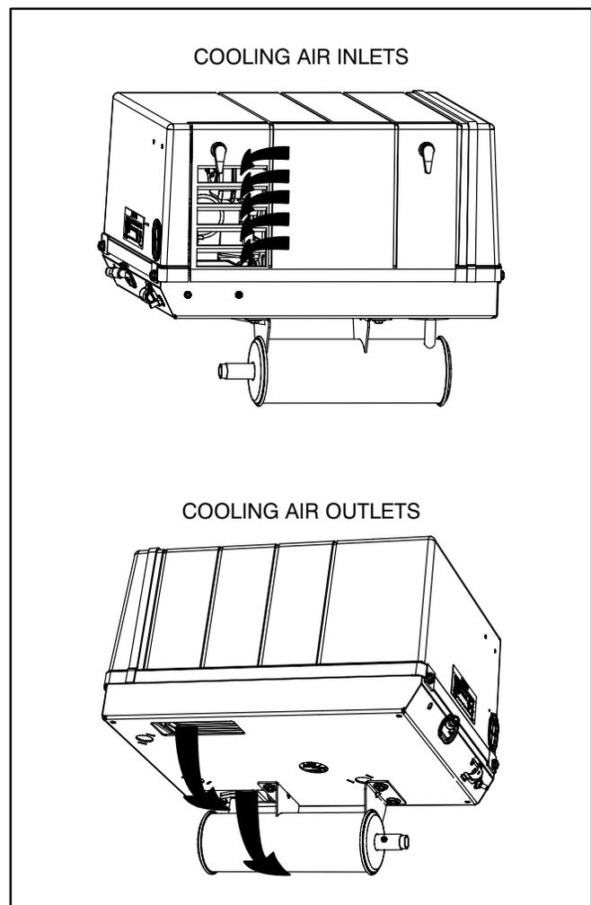
FIGURE 8-2. MODEL KYD COOLING AIRFLOW
