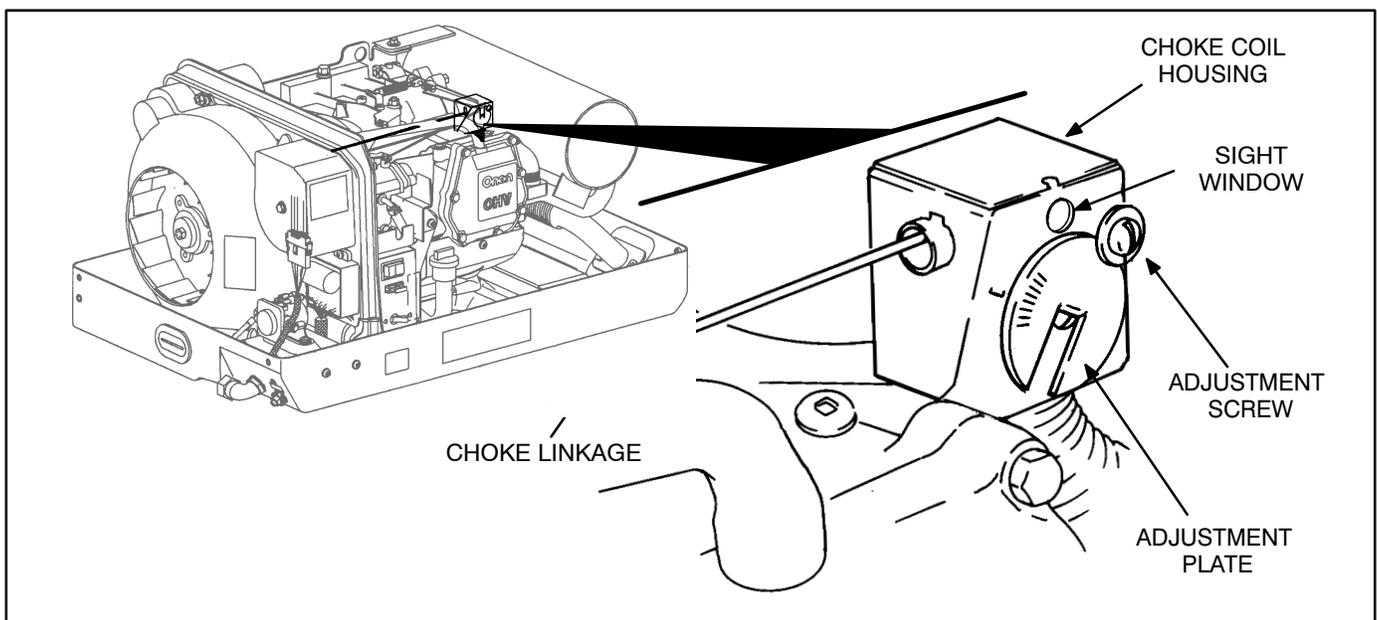
FIGURE 8-10. CHOKE ASSEMBLY
