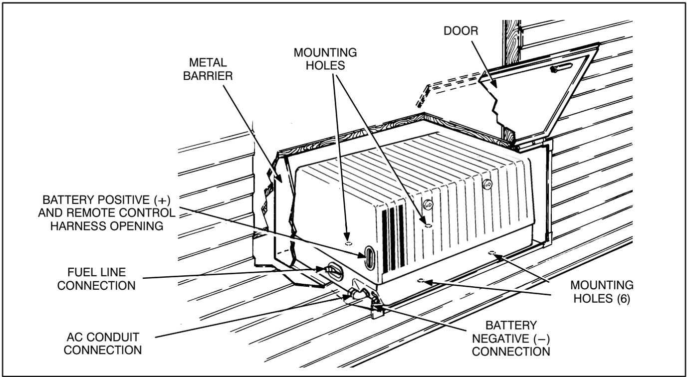
**FIGURE 5-1. TYPICAL COMPARTMENT MOUNT INSTALLATION**
