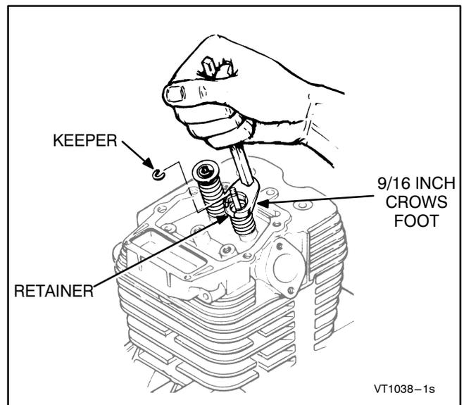
**FIGURE 9-7. VALVE REMOVAL**
