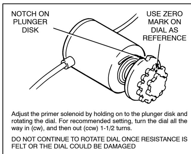
**FIGURE 8-14. AUTOMATIC PRIMING SOLENOID (PRIOR TO SPEC L (MODEL KY) OR SPEC B (MODEL KYD))**
