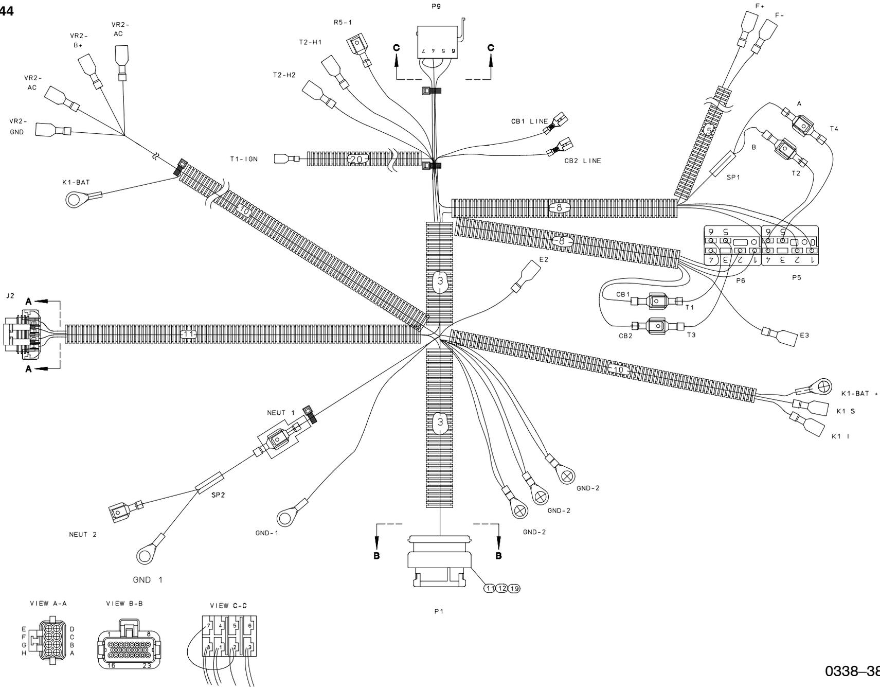
ENGINE WIRING HARDNESS—50 HERTZ AND 60 HERTZ, 100V
