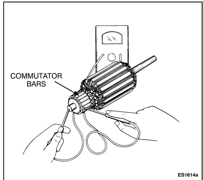
FIGURE 8-19. TESTING ARMATURE FOR GROUNDS
