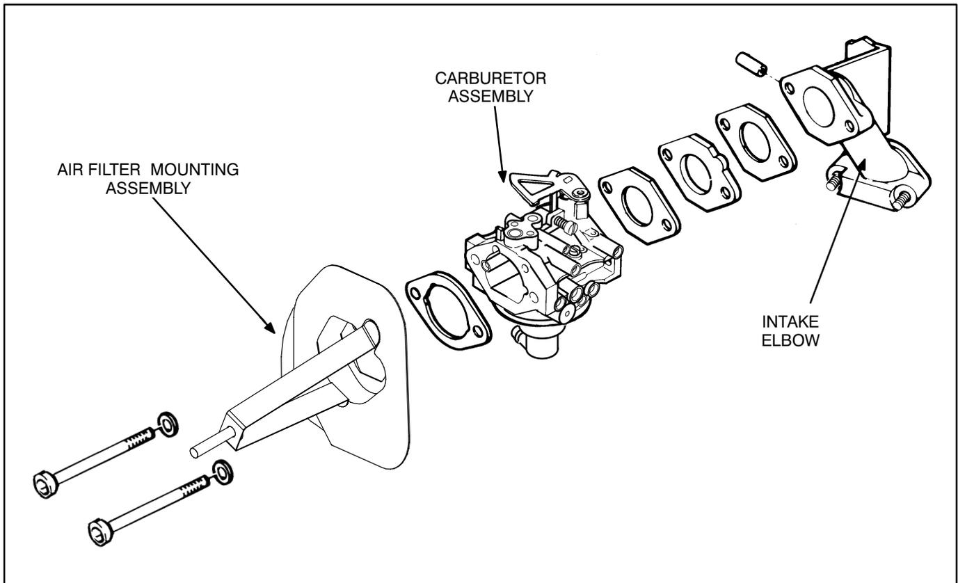
FIGURE 8-8. CARBURETOR AND INTAKE MANIFOLD ASSEMBLY
