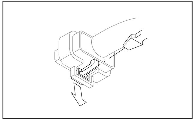
FIGURE 6-3. DISCONNECTING P1
