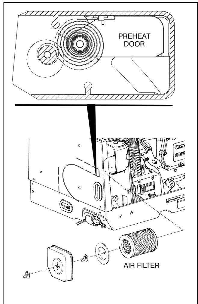
**FIGURE 8-7. AIR FILTER AND PREHEATER ASSEMBLY**
