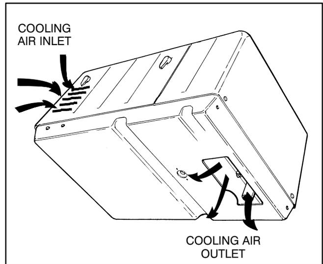
FIGURE 8-1. MODEL KY COOLING AIRFLOW
