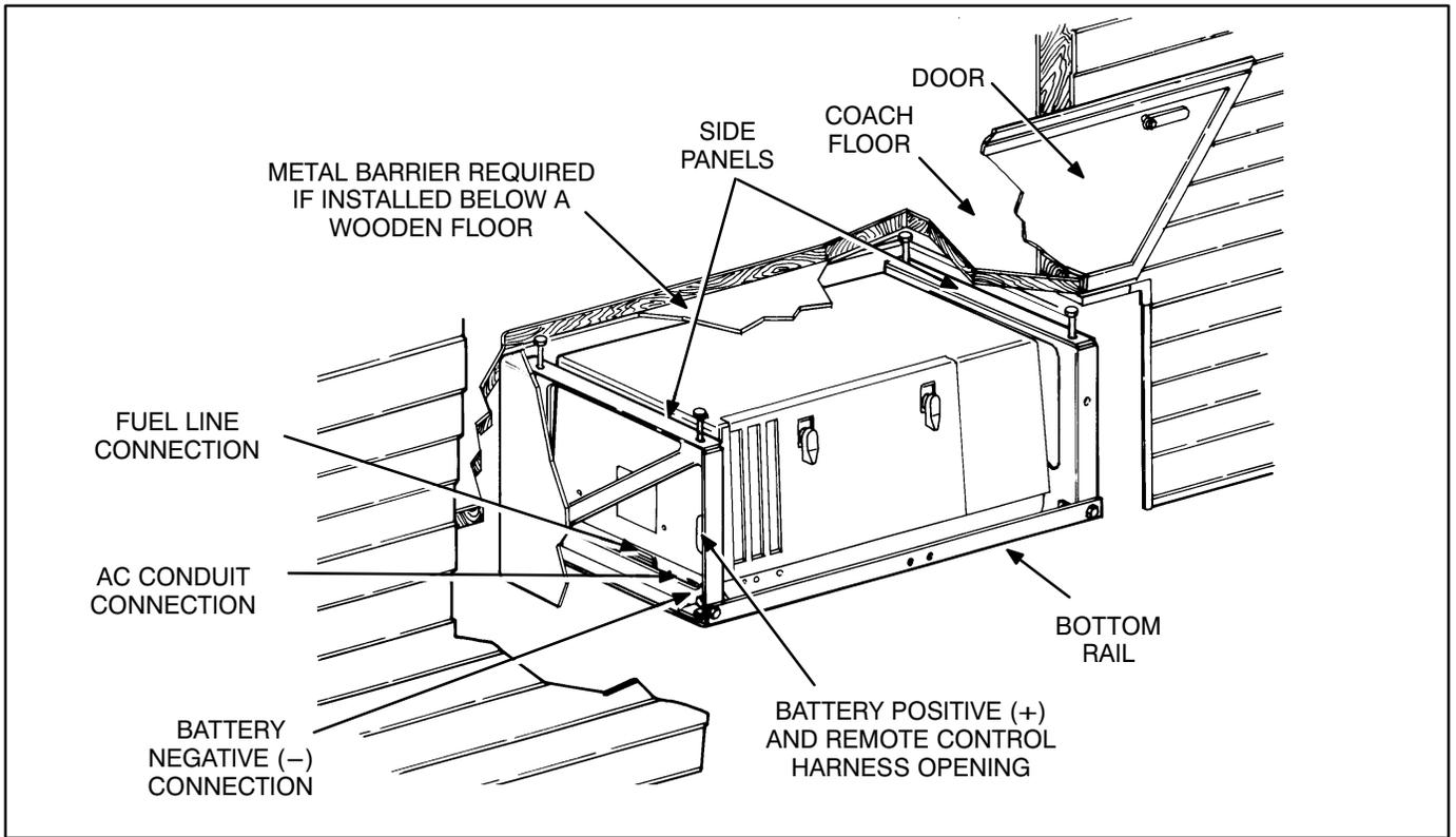
**FIGURE 5-2. TYPICAL UNDER-FLOOR MOUNT INSTALLATION**
