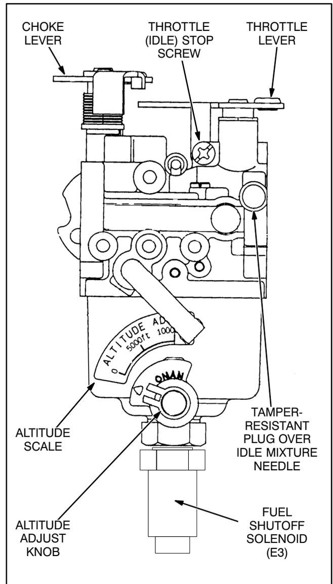
**FIGURE 8-9. CARBURETOR ADJUSTMENTS**
