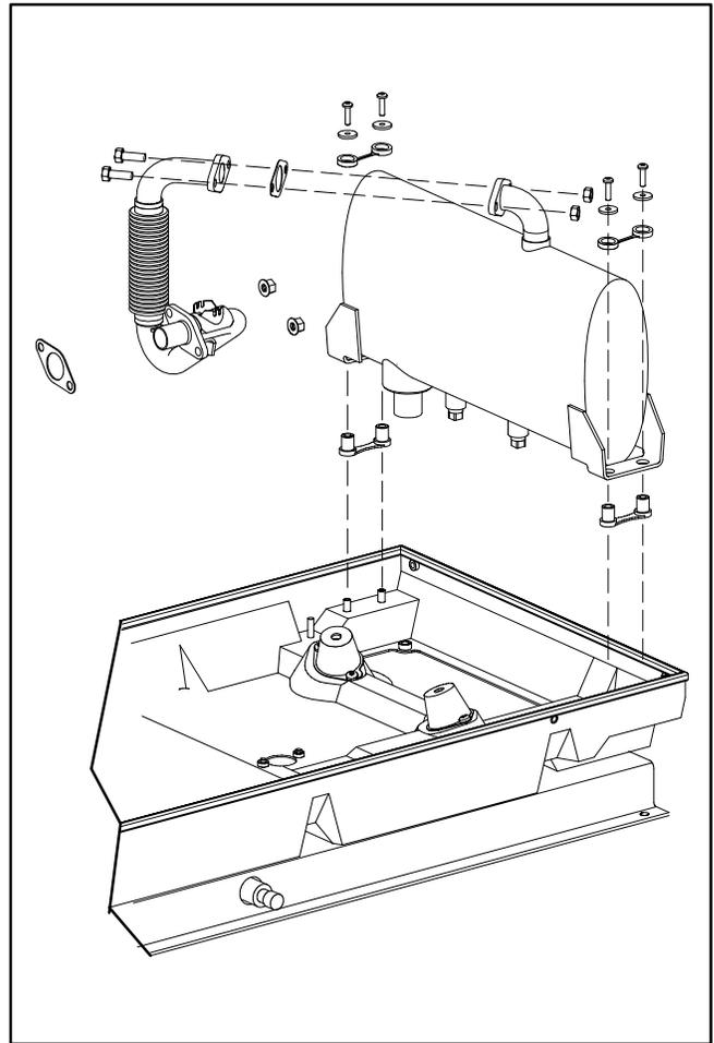
FIGURE 8-3. MODEL KY MUFFLER
