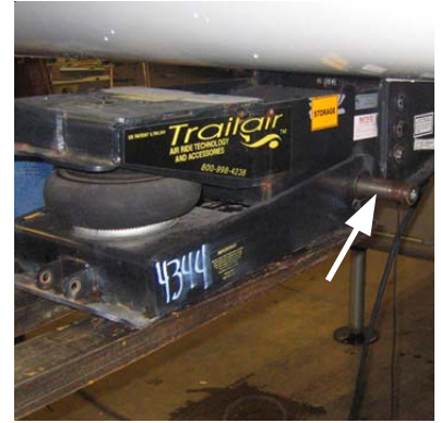
Remove lower jaw pivot pin.
