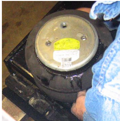
Set old lower jaw aside and place the Tri-Glide lower jaw in it's place. Mount airbag. Place bolt head in hole and slide into place.
