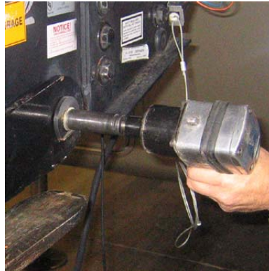
Remove lower jaw pivot bolts and washers on both sides.
