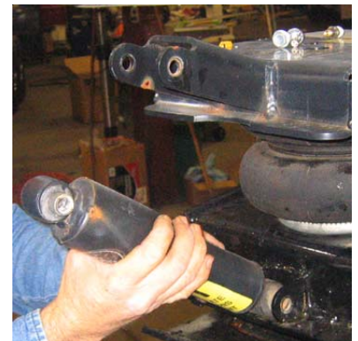
Install shock, do not tighten bolts yet.
