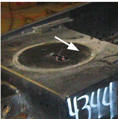
Remove lower jaw slowly, jaw is heavy. Works best by simply lowering forks of the forklift. Slide airbag over and disengage.
