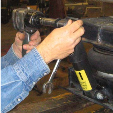
Disengage shock bolts and remove shock.
