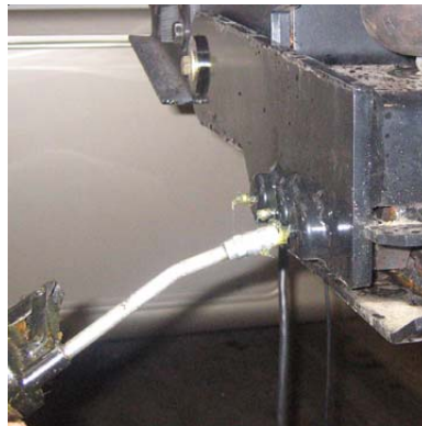
Grease all zerks, there are a total of 9; 3 on each side of the Tri-Glide jaw...
