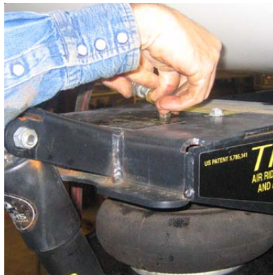
Fill airbag. Test airbag for leaks using soapy water procedure.
