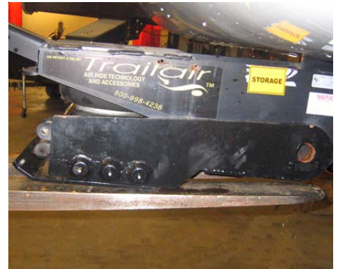
Lift Tri-Glide jaw into place.
