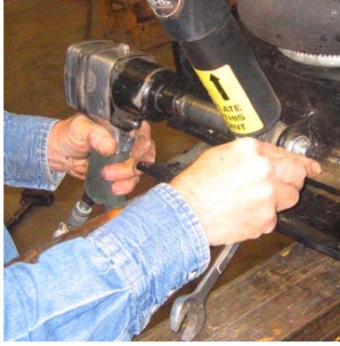
Tighten shock mounting bolts. Torque bolts 90 - 110 ft. lb.
