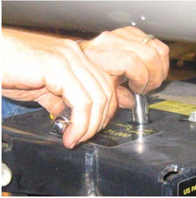
Replace air valve and air bag mounting bolts, tighten into place.
