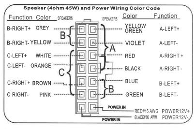
. Pay attention to the wiring connection: Wrong connection or reverse polarity (+/-) can cause distortion
