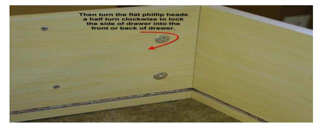
After putting together one side panel with the front and back panels, it is time **to install the bottom of the drawer**. Slide the bottom panel into the slotted groove between the front and back panels, then into the one side panel. Make sure that the sticker is up and towards the front of the kickboard. Then, install the other side panel (making sure that the open end of the slide track is toward the back drawer panel), and turn the other flat-Phillips screws ½ turn clockwise.
