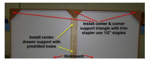
Install L brackets on the back of the kickboard and connect them to the out side of the drawer end panels. Then, install the drawer to the backside of the kickboard using the predrilled holes in the backside of the drawer panel. Now slide the drawer into the bottom of the sofa.
