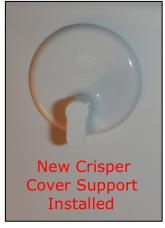
mine. I assume it broke from the weight of the contents of the drawer and shelf above it, combined with the bounce of the road.
