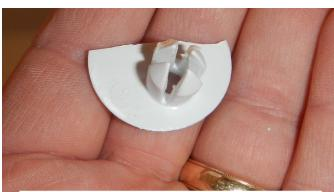
EXAMPLE OF BACK SIDE OF BROKEN PART NOTE HOW BARBS EXPAND WHEN PIN IS PUSHED IN
